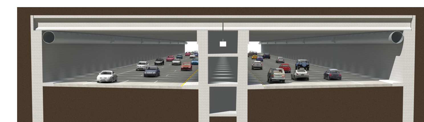
Cut and Cover Tolled Express Tunnel
