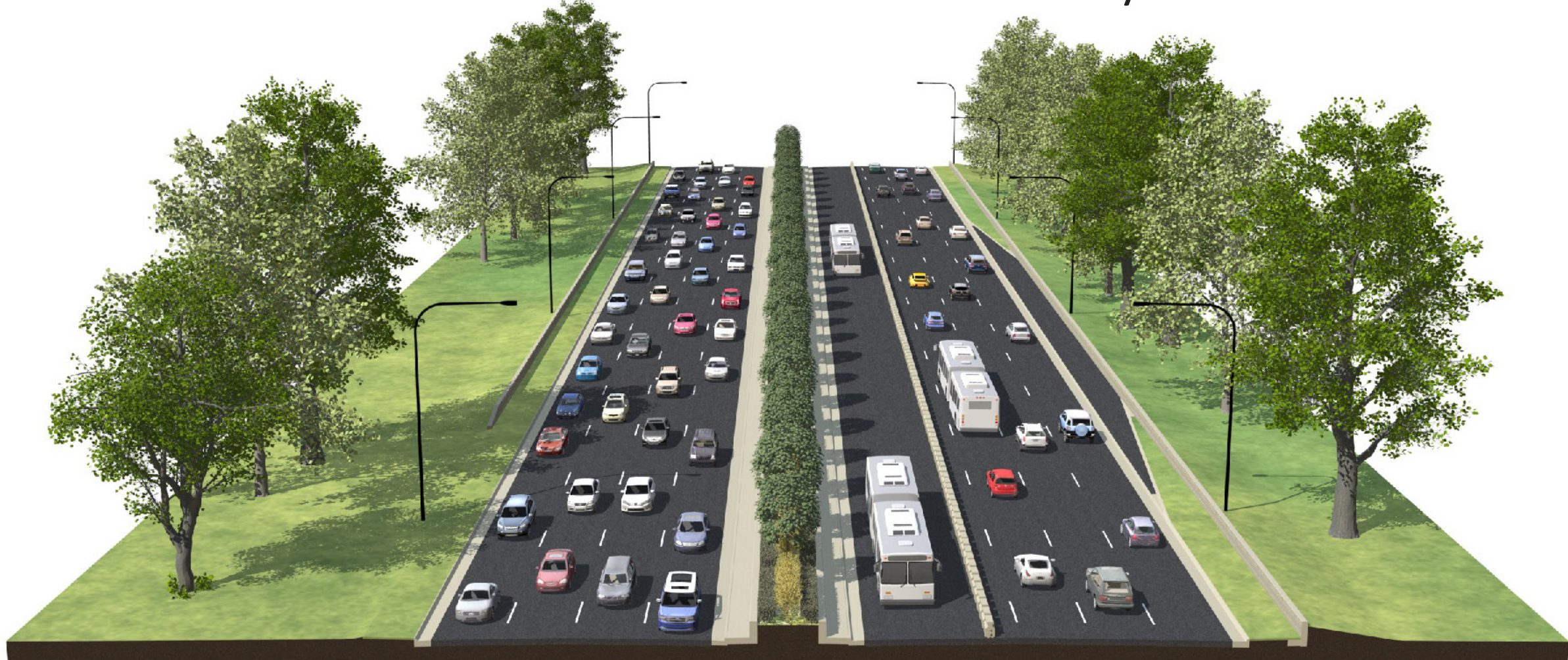
Four-Plus-One Contraflow SB Bus-Only Lane
