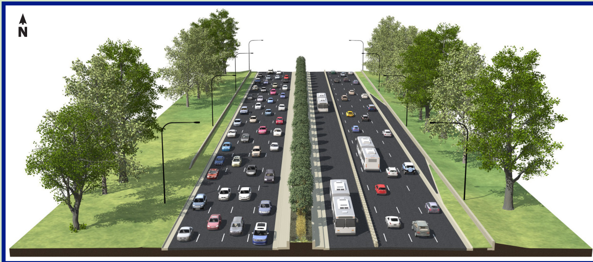
Converts the left NB GPL to a one-way SB BOL for the AM peak period
