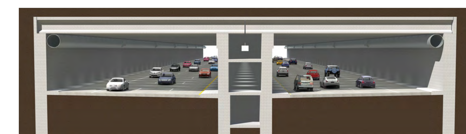
Cut and Cover Tolled Express Tunnel
